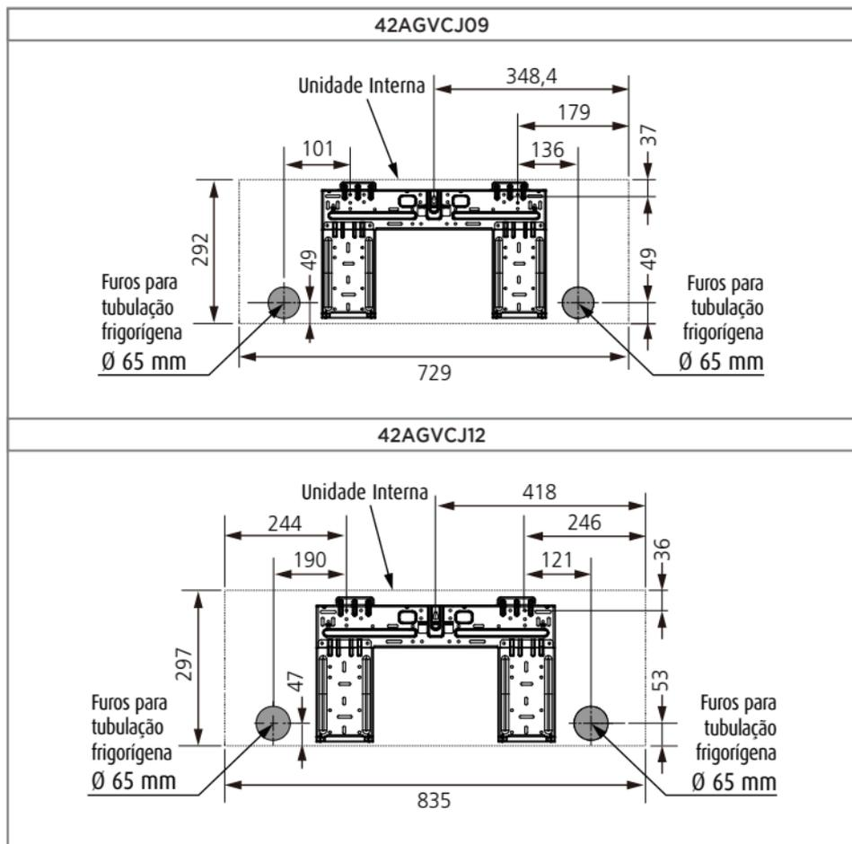
FIG. 11 - PLACAS DE MONTAGEM
