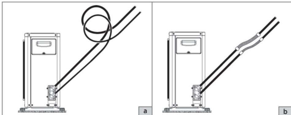
FIG. 13 - LOOP'S E TUBOS FLEXÍVEIS
