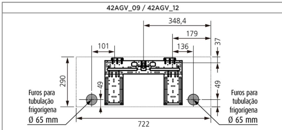
FIG. 11-A - PLACAS DE MONTAGEM
