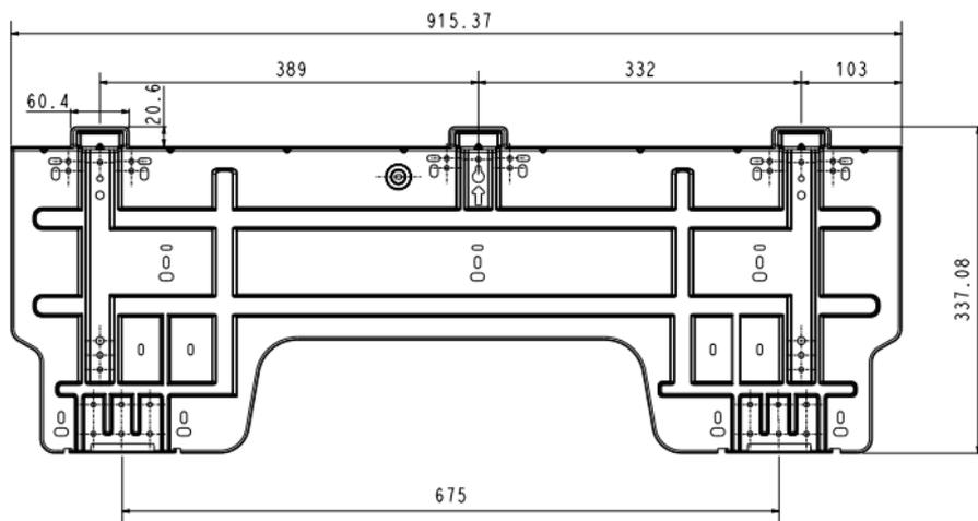
FIG. 11-B - PLACAS DE MONTAGEM
