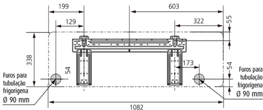
FIG. 11 - PLACAS DE MONTAGEM
